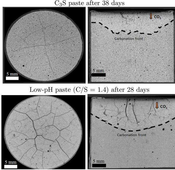
Figure 2:  $\mu$ CT scan of samples subjected to accelerated carbonation (voxel size =  $17 \mu\text{m}$ ). Left panel: top view of the sample, right panel: transverse view of the sample. These scans show the evolution of the carbonation front as well as the appearance of cracks. Measurement of the extent of the carbonation front were coupled with XRD profiles, thermogravimetric analysis and phenolphthaleine tests.
