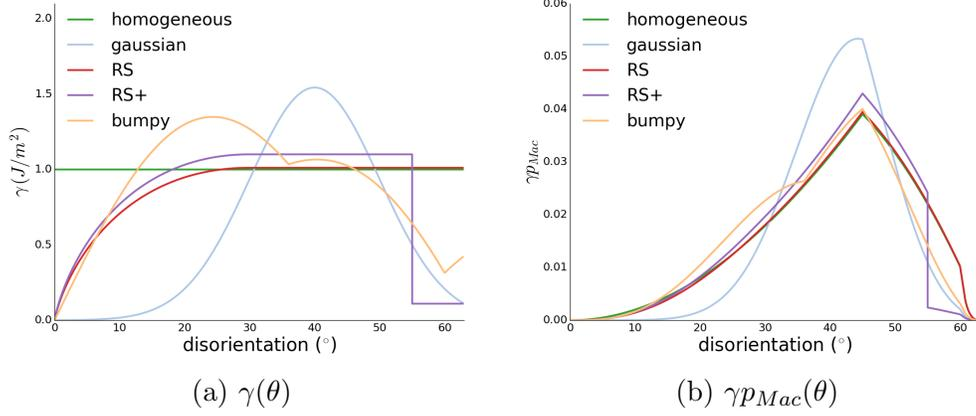
Figure 7: Considered test grain boundary energy functions.
