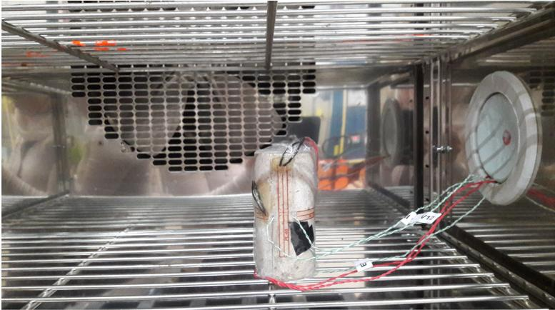
(a) The specimen inside the environmental chamber.
