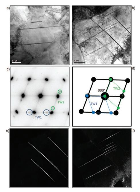
Fig. 2. TEM images illustrating the early twinning activity: (a) mechanical twins after 0.02 true strain, (b) two non coplanar twin systems after 0.05 true strain, corresponding (c) experimental and (d) simulated selected area electron diffraction patterns (the spots corresponding to each twin system are labelled TW1 and TW2, respectively) and (e and f) corresponding dark field images.
