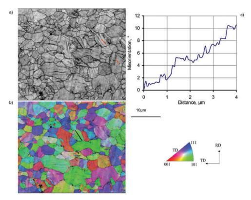
Fig. 4. EBSD maps of sample strained to 0.1 true strain: (a) KPQ map, (b) TD-IPF map and (c) cumulative misorientation profile along the black line drawn on the maps.
