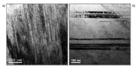
Fig. 5. TEM bright field image of twins after 0.3 true strain. (a) Global and (b) detailed view of the twin bundles.
