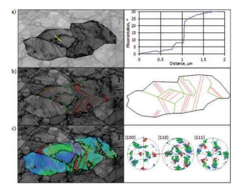
Fig. 10. Different EBSD representations corresponding to the grain marked by the white star in Fig. 7. (a) KOP map with the misorientation profile along the vellow line. (b) KPO map with specific misorientation lines and corresponding schematic drawings; twin boundaries in red – grain boundaries misoriented by less than  $3^{\circ}$  in white and less than  $10^{\circ}$  in green and (c) TD-IPF map with the corresponding  $\{100\}$ ,  $\{110\}$ , and  $\{111\}$  pole figures.
