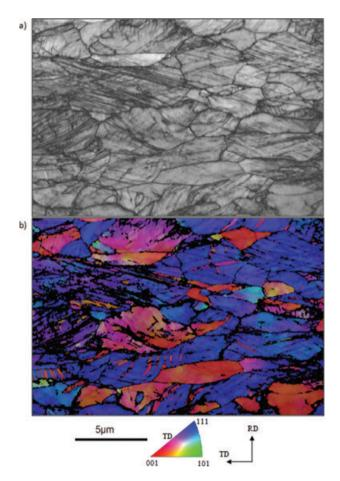
Fig. 11. EBSD maps of sample strained to 0.4 true strain: (a) KPQ map and (b) TD-IPF map.
