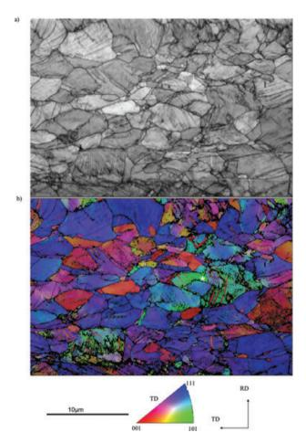
Fig. 7. EBSD maps of sample strained to 0.3 true strain: (a) KPQ map and (b) TD-IPF map.
