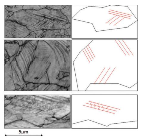
Fig. 8. KPQ maps highlighting specific grains with different twin configurations.
