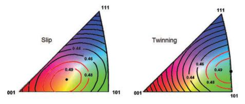
Fig. 9. Iso-density lines of maximum Schmid factors (a) for slip and (b) twinning plotted in the unit triangle of the TD-IPF (the IPF orientation colour code is also given in semi-transparency).
