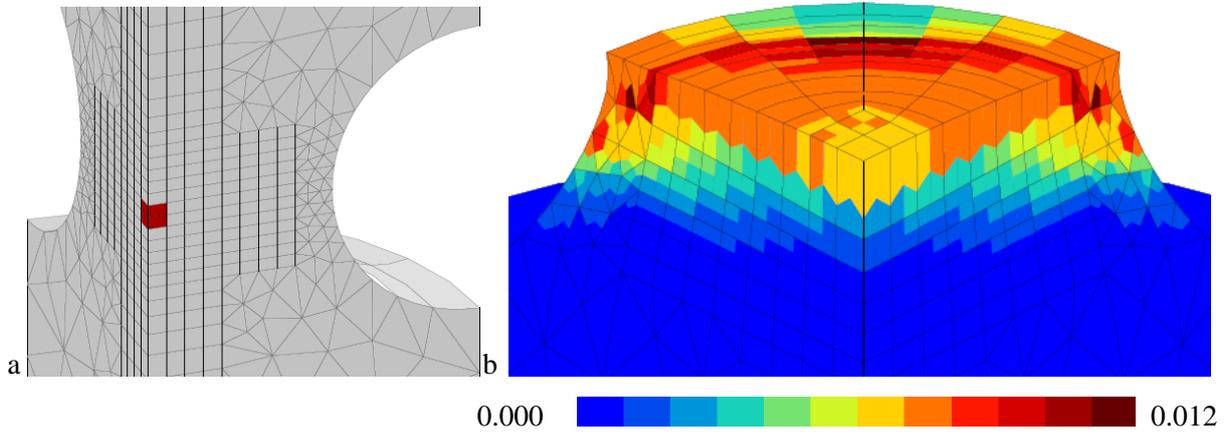
Figure 4. AE4 notched tensile specimen,  $f_0 = 0.0001$  (small sulfur content) : a) Cartesian mesh in the specimen minimum section, b) volume fraction of carbides with nucleated submicron voids in the broken specimen, 0.006-0.007 in the center, light orange color, nucleated fraction  $\cong 25\%$  [21]. The layer of broken integration points is strongly stretched in the vertical direction, it corresponds to crack opening.
