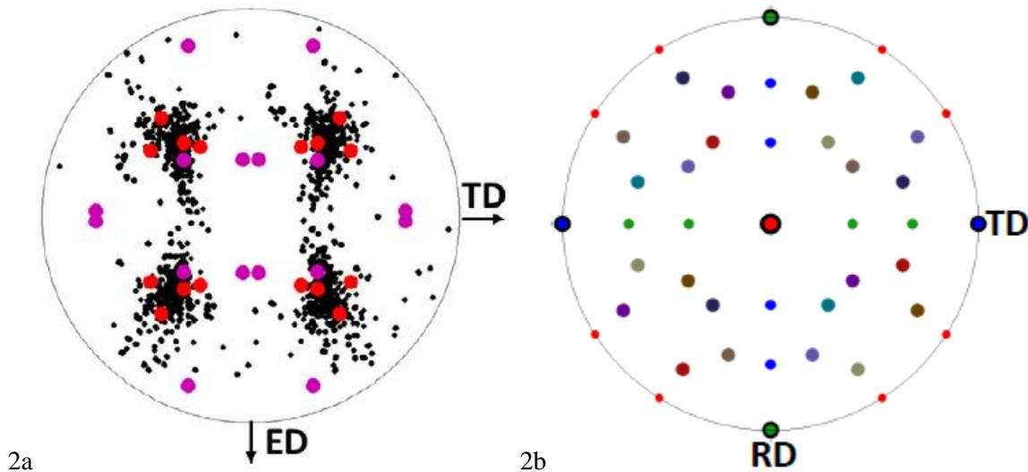
Figure 2. a)  $\{111\}$  pole figure of a 6260-T6 aluminum alloy extrusion (1 mm thickness central layer), black discs: EBSD measurements, colored discs: orthotropic texture reduced to 8 orientations. b)  $\{100\}$  pole figure, equal area projection, "isotropic" reduced texture with 15 orientations.
