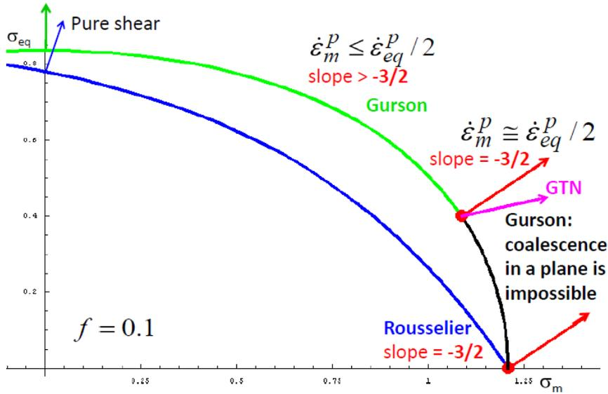
Figure 1. Yield surfaces in porous plasticity with  $f=0.1$ ,  $\sigma_p=1$ . Modified Gurson model with  $q_1=1.6245$ ,  $q_2=1$ ,  $q_3=2.25$  (green and black curves). Rousselier model with  $\sigma_1=(2/3)\sigma_p$  and  $D_1=2$  (blue curve). Red arrows (plastic flow direction) correspond to the NKCML, Eq. (3<sub>1</sub>). Effect on plastic flow direction of the GTN model void growth acceleration function with  $K=\delta=3$ , loss of normality.
