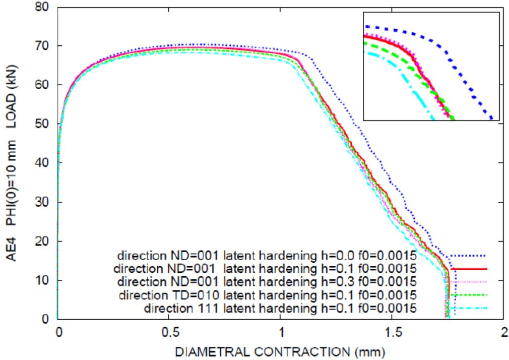
Figure 6. Load-displacement curves of the AE4 notched tensile specimen ( $f_0 = 0.0015$ ). Latent hardening effect (ND tensile direction), tensile direction effect (for  $h = 0.1$ ). All curves without secondary voids ( $f_{N2} = 0$ ).
