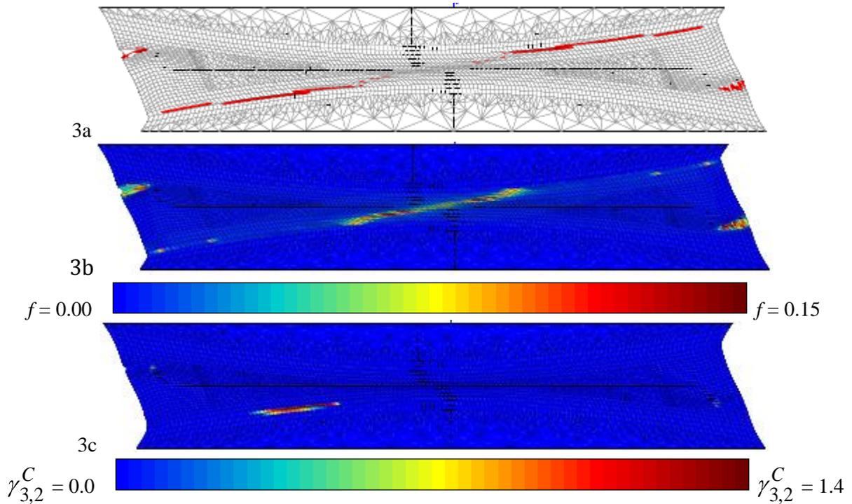
Figure 3. 6260-T6 aluminum alloy shear specimen : a) time=404, crack at mid-thickness ("broken" integration points in red), b) time=404, void volume fraction  $f$ , c) time=320, left: "Coulomb" cumulated slip ( $g = 3, s = 2$ ), the slip system ( $g = 2, s = 12$ ) forms a symmetric crack on the right (not shown in the figure) [8].
