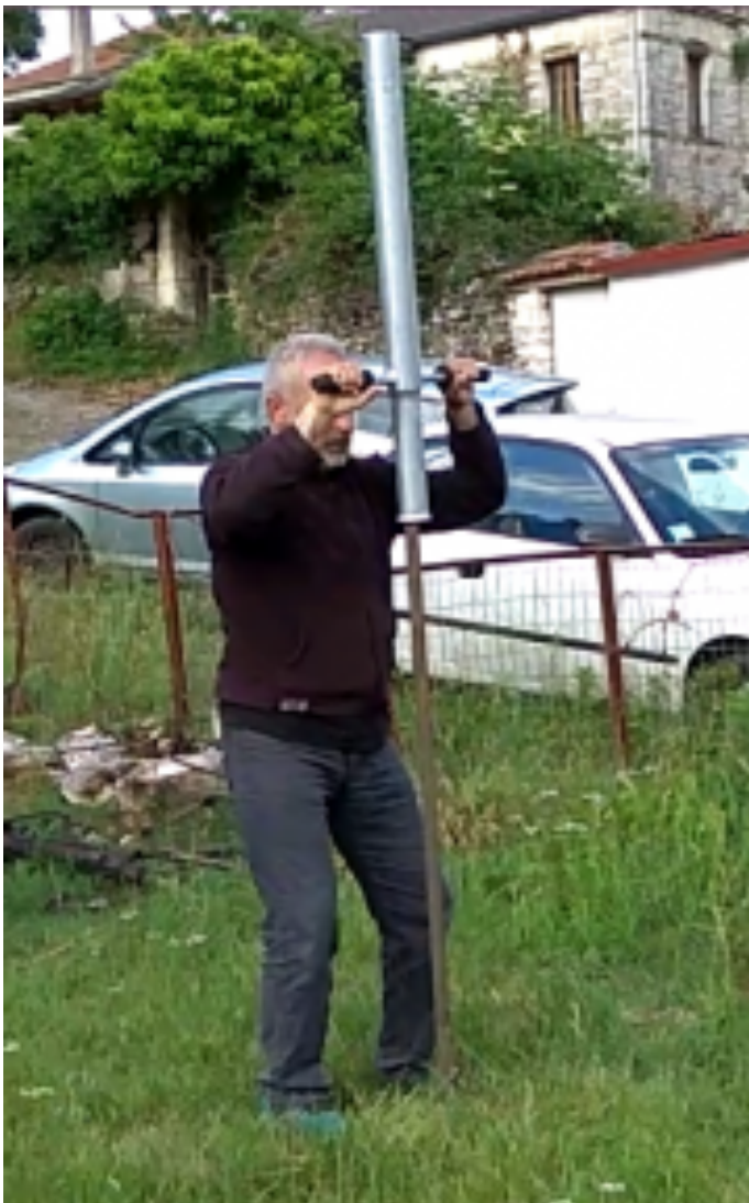
Picture 4: Testing the newly constructed tool for hammering fencing-poles from the Tzoumakers group. Source: Alekos Pantazis.
