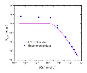
**Fig. 10.** Experimental (blue squares) and modeled (magenta line) dissociation constants for Cs<sup>+</sup> in mineral water as a function of the equilibrium Cs<sup>+</sup> concentration for powdered silica monoliths functionalized with Cu/K hexacyanoferrate nanoparticles (powdered HCF@silica-monolith).
