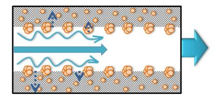
**Fig. 6.** Simplified model of reactive transport for Cs<sup>+</sup> in a macroporous channel in silica monoliths functionalized with hexacyanoferrate nanoparticles (orange circles); the dispersion inside the macroporous channel is derived from the dispersion of the monolithic structure.
