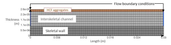
**Fig. 7.** Modeling grid used for the reactive transport of Cs<sup>+</sup> ions in silica monoliths functionalized with Cu/K hexacyanoferrate nanoparticles (HCF@silica-monolith); the dispersion of solute transport in the channel was fitted from the RTD experiments to take into account the tortuosity of the silica monolith; diffusion was only allowed in the aggregate and skeletal wall.
