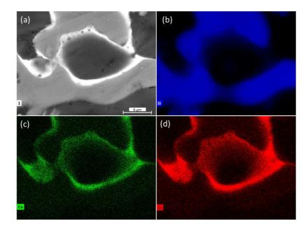
**Fig. 4.** (a) Scanning electron micrograph of a polished cross section of a Cu/K-hexacyanoferrate–functionalized silica monolith (HCF@silica-monolith) after a cesium sorption experiment and (b–d) corresponding energy-dispersive X-ray maps for silicon (blue), copper (green) and cesium (red).
