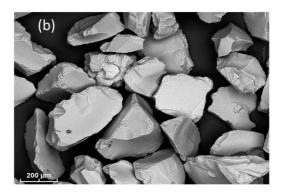
**Fig. 1.** Scanning electron micrographs of (a) crushed monolithic silica gel (200–500  $\mu$ m in diameter) and (b) commercial silica gel particles (also 200–500  $\mu$ m in diameter).
