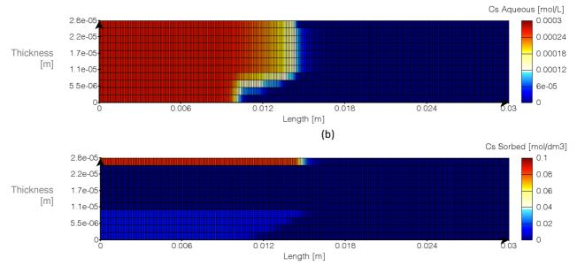
**Fig. 15.** (a) Aqueous and (b) sorbed concentrations of Cs<sup>+</sup> in the different regions of the reactive transport model of a silica monolith functionalized with Cu/K hexacyanoferrate nanoparticles (HCF@silica-monolith) after 6 min of a breakthrough experiment at a Darcy velocity of 8 m·h<sup>-1</sup>. The sorbed concentrations are given per dm<sup>3</sup> of pore volume.
