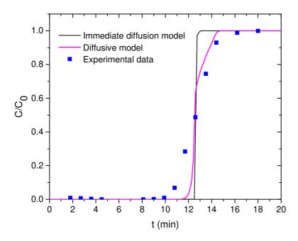
**Fig. 14.** Reactive transport modeling of the Cs<sup>+</sup> breakthrough curve for a silica monolith functionalized with Cu/K hexacyanoferrate nanoparticles (HCF@silica-monolith) a Darcy velocity of 8 m·h<sup>-1</sup>. The curve obtained with a model assuming immediate diffusion to all the HCF nanoparticles in the monolith is shown for comparison.
