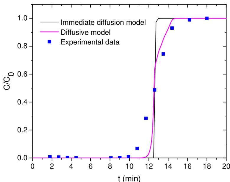
**Fig. 14.** Reactive transport modeling of the  $\text{Cs}^+$  breakthrough curve for a silica monolith functionalized with Cu/K hexacyanoferrate nanoparticles (HCF@silica-monolith) at a Darcy velocity of  $8 \text{ m}\cdot\text{h}^{-1}$ . The curve obtained with a model assuming immediate diffusion to all the HCF nanoparticles in the monolith is shown for comparison.
