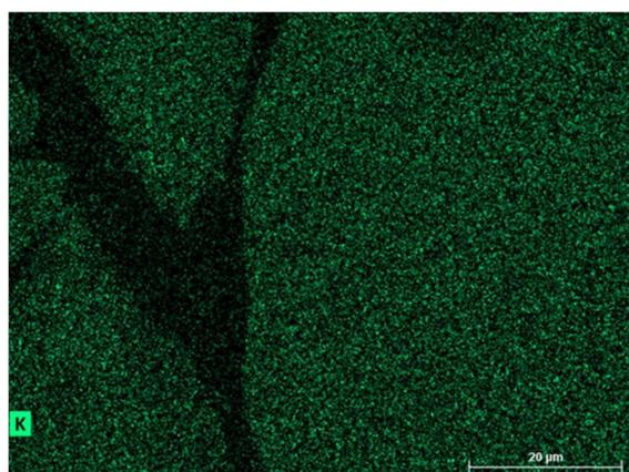
**Fig. 5.** Energy-dispersive X-ray map of potassium (in green) in a polished cross section of a packed sample of commercial silica gel particles functionalized with Cu/K hexacyanoferrate set in epoxy resin.
