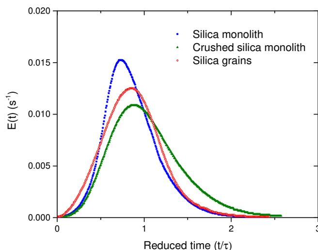
**Fig. 11.** Residence time distributions measured for columns packed with a silica monolith (blue), crushed silica monolith (green), and commercial silica gel particles (red) at a Darcy velocity of  $0.8 \text{ m}\cdot\text{h}^{-1}$  ( $[\text{NaNO}_3]_0 = 10.0 \text{ g}\cdot\text{L}^{-1}$ ).
