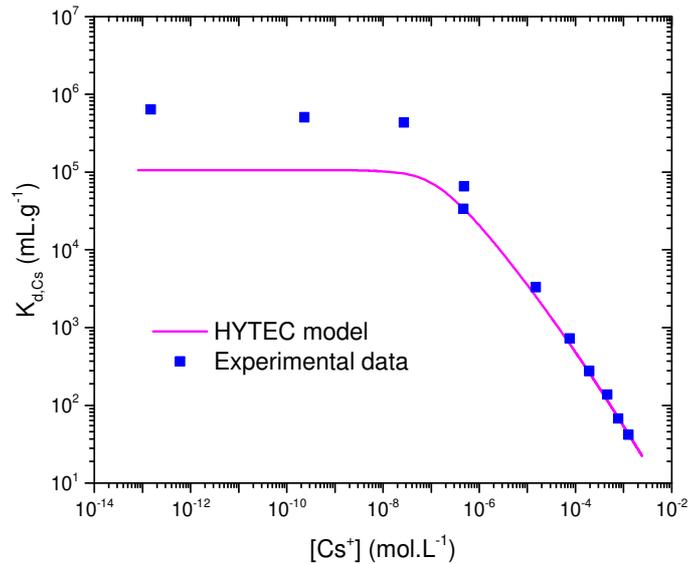
**Fig. 10.** Experimental (blue squares) and modeled (magenta line) dissociation constants for Cs<sup>+</sup> in mineral water as a function of the equilibrium Cs<sup>+</sup> concentration for powdered silica monoliths functionalized with Cu/K hexacyanoferrate nanoparticles (powdered HCF@silica-monolith).
