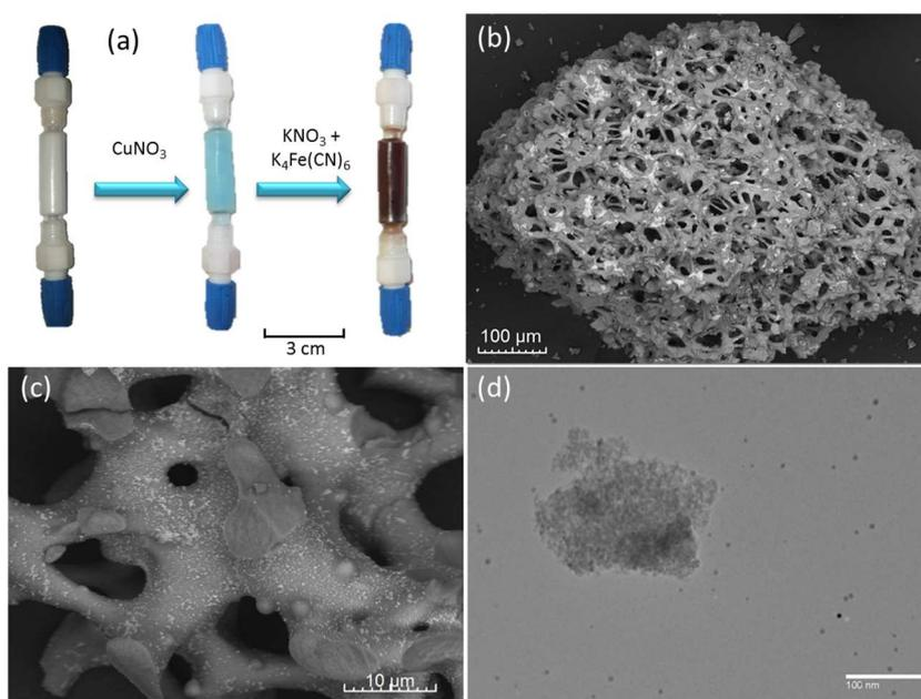
**Fig. 3.** Hierarchical porous silica monolith functionalized with Cu/K hexacyanoferrate (HCF@silica-monolith): (a) photographs of a monolith at different stages of the functionalizing process, (b) scanning electron micrograph of the macroporous network, (c) scanning electron micrograph of HCF aggregates deposited on the surface of the skeletal walls, and (d) transmission electron micrograph of an aggregate of HCF nanoparticles.
