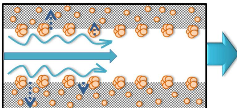
**Fig. 6.** Simplified model of reactive transport for  $\text{Cs}^+$  in a macroporous channel in silica monoliths functionalized with hexacyanoferrate nanoparticles (orange circles); the dispersion inside the macroporous channel is derived from the dispersion of the monolithic structure.
