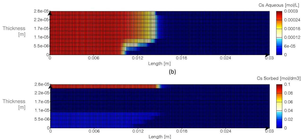
**Fig. 15.** (a) Aqueous and (b) sorbed concentrations of Cs<sup>+</sup> in the different regions of the reactive transport model of a silica monolith functionalized with Cu/K hexacyanoferrate nanoparticles (HCF@silica-monolith) after 6 min of a breakthrough experiment at a Darcy velocity of 8 m·h<sup>-1</sup>. The sorbed concentrations are given per dm<sup>3</sup> of pore volume.
