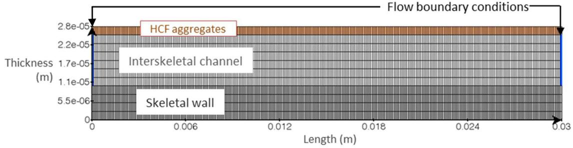
**Fig. 7.** Modeling grid used for the reactive transport of  $\text{Cs}^+$  ions in silica monoliths functionalized with Cu/K hexacyanoferrate nanoparticles (HCF@silica-monolith); the dispersion of solute transport in the channel was fitted from the RTD experiments to take into account the tortuosity of the silica monolith; diffusion was only allowed in the aggregate and skeletal wall.
