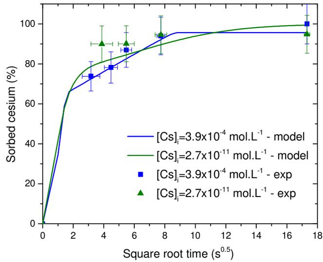
**Fig. 9.** Reactive transport modeling (Figs. 7 and A.2, Table 1) of the sorption kinetics of powdered silica monoliths functionalized with Cu/K hexacyanoferrate nanoparticles (powdered HCF@silica-monolith) for  $\text{Cs}^+$  in mineral water at  $3.9 \times 10^{-4} \text{ mol}\cdot\text{L}^{-1}$  ( $^{133}\text{Cs}^+$ , blue) and at a trace concentration ( $^{137}\text{Cs}^+$ , green). The experimental data are shown as points with error bars.
