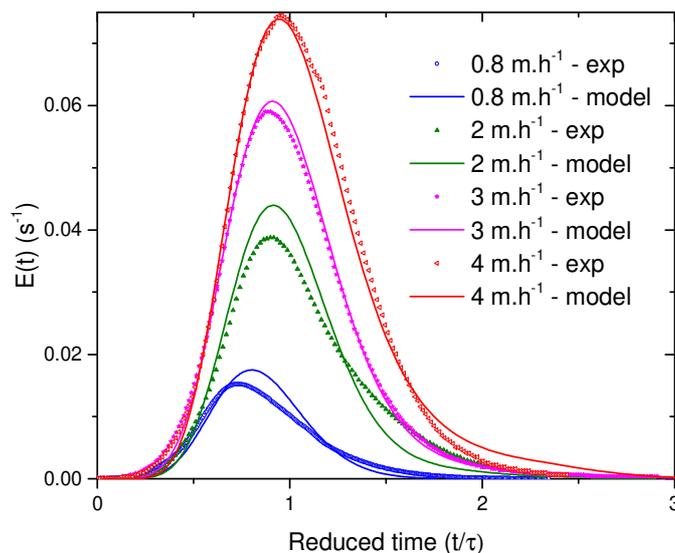
**Fig. 12.** Residence time distributions (time normalized to the ideal residence time) measured for silica monoliths at increasing Darcy velocities and the corresponding best fits calculated by reactive transport modeling (Figs. 7, Table 1).
