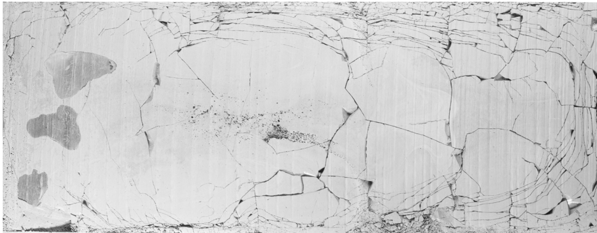
Figure 2 Grayscale image of the UMo bloc of nuclear fractured glass. Dimensions: 1044 mm × 413 mm.
