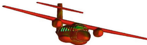
Fig. 1. Surface currents on an aircraft model from a boundary element simulation with around 2 million unknowns.
