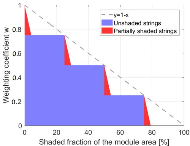
Figure 12: Illustration of the evolution of the weighting factor  $w$  with the shaded fraction of the module area  $f_{shading}$ , in the example of four parallel strings with 6x12 cells panel in landscape (same example as 19 B. The violet part corresponds to the contribution of the unshaded strings, the red part corresponds to the contribution of the partially shaded one.
