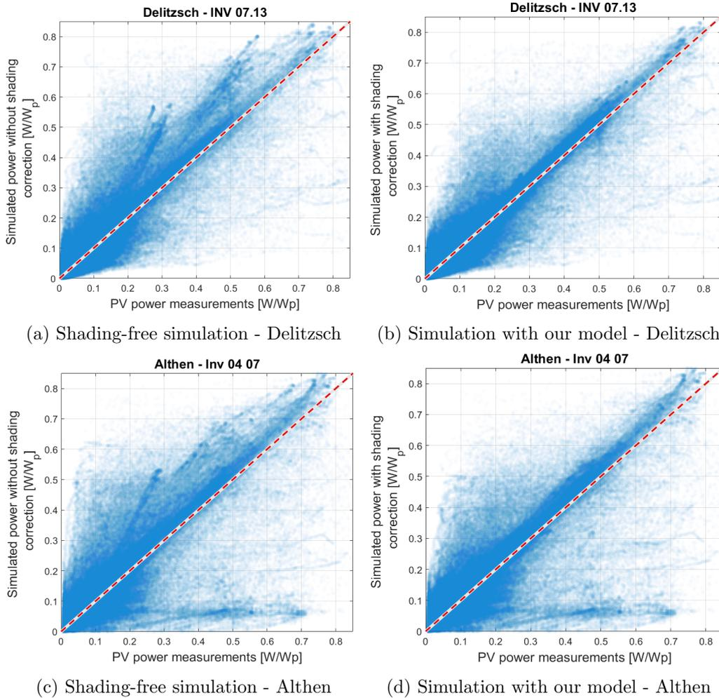
Figure 13: Comparison of the simulated power values (ordinate) against the corresponding measurements (abscissa) with and without consideration of the inter-row shading (left and right plots respectively) and for the Delitzsch and Althen PV plants (upper and lower plots respectively).
