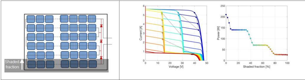
(c) Effect of a partial shading on the power output of a landscape oriented PV module with three bypass diodes
