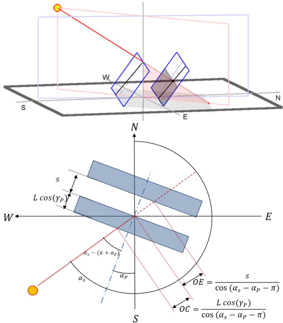
Step 3: Calculation in the plane including the sun and the vertical at the origin (light red).
