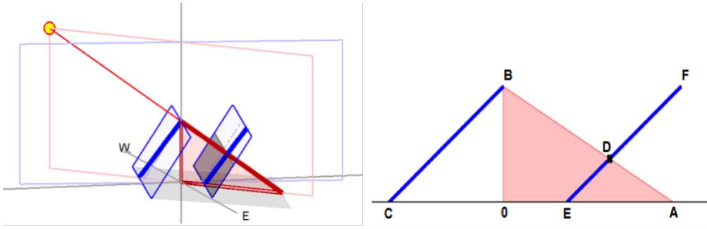
Figure 6: Illustration of the lengths used for the calculation of the shaded fraction in the space (left) and in the plane including the sun and the origin (right).
