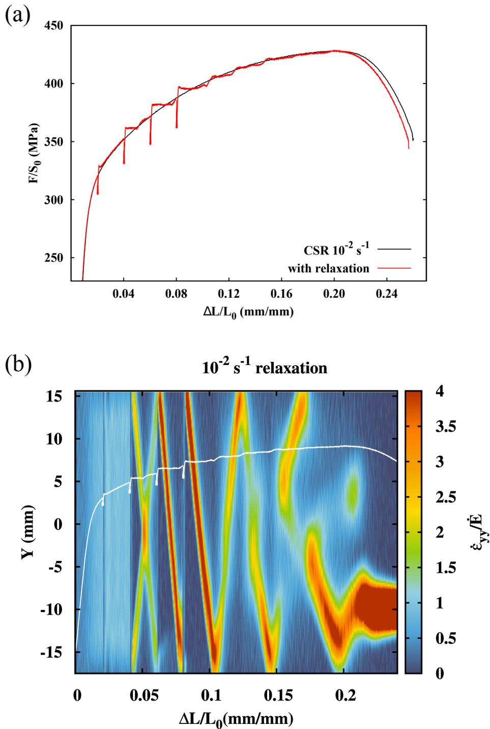
Figure 3: (a) Constant strain rate tensile test at a strain rate  $10^{-2} \text{ s}^{-1}$  (black line) superposed with the curve of tensile test including relaxations. (b) The experimental spatio-temporal pattern of the relaxation test at a strain rate  $10^{-2} \text{ s}^{-1}$  ( $\Delta t = 0.05 \text{ s}$ ).
