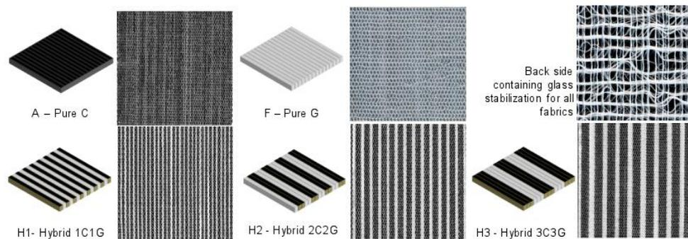
**Figure 1.** Schematic and pictures of the fabrics manufactured.
