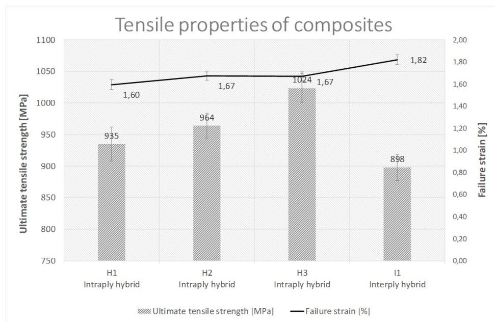
**Figure 2.** Tensile properties of manufactured hybrid composites.
