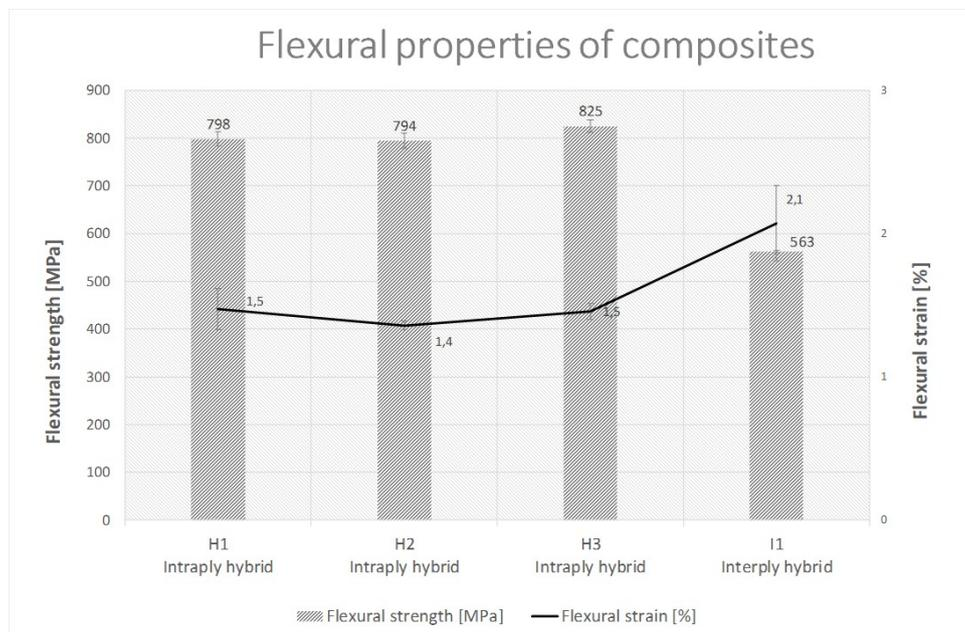
**Figure 3.** Flexural properties of manufactured hybrid composites.
