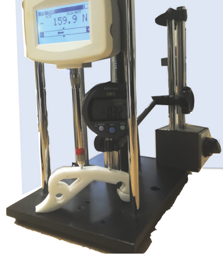
FIGURE 2: Experimental setup. A mechanical load of 159.9 N is applied on the top of the part in white. A displacement is measured at a fixed point.
