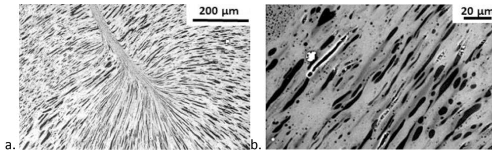
**Figure 9:** Morphology pattern of the ternary blend 60PLA/20PBAT<sub>1</sub>/20PA at the diverging entrance of the recirculating reservoir in the micro-compounder (180°C, 80 rpm, 12 min): a. overall view; b. enlargement of a zone showing the twinning of PA (black) and PBAT (dark gray) phases.
