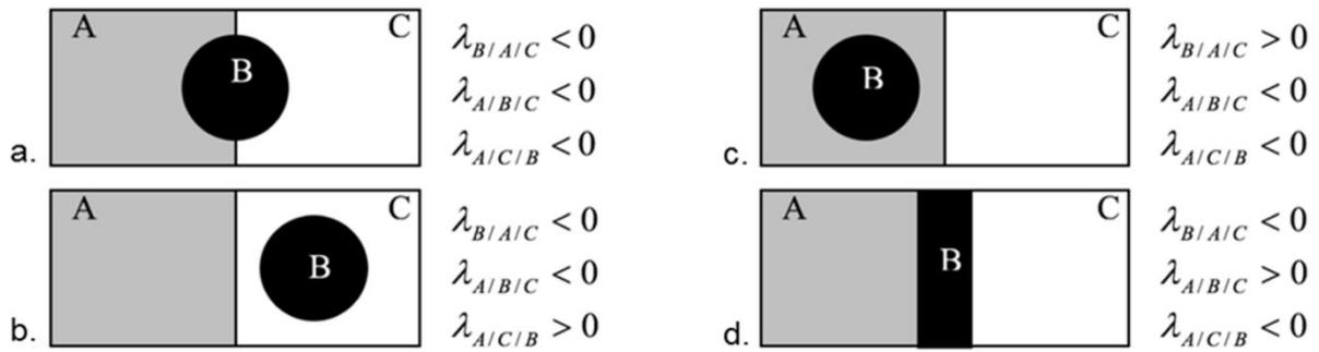
**Figure 1:** Four possible equilibrium morphologies for a ternary polymer blend, with a minor phase C and two major phases A and B, and their relations to the respective signs of the spreading coefficients, according to reference <sup>9</sup>.
