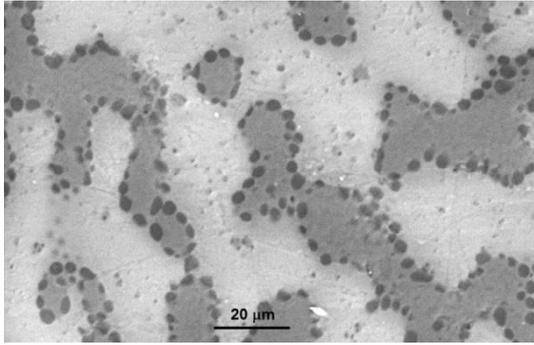
**Figure 6:** SEM micrograph of a 60PLA/27PBAT<sub>1</sub>/13PA ternary blend prepared in the internal mixer: at 180°C, 50 rpm for 12 min. The black phase is PA, the dark gray phase is PBAT<sub>1</sub> and the light gray phase is PLA.
