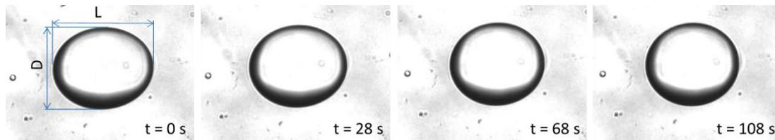
**Figure 3:** Relaxation of an ellipsoidal drop of PBAT<sub>1</sub> in the PLA matrix after deformation under shear (flow direction is horizontal, vorticity axis is vertical). The drop radius is 83 μm.
