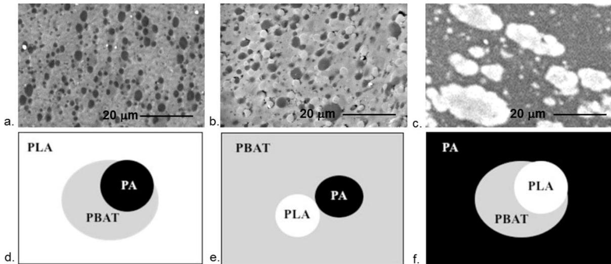
**Figure 7:** Morphologies of the three blends: a. 60PLA/20PBAT<sub>2</sub>/20PA; b. 60PBAT<sub>2</sub>/20PA/20PLA and c. 60PA/20PLA/20PBAT<sub>2</sub> as seen by SEM and their respective model predictions (d. to f.). Blends were prepared in the internal mixer at 180°C, 80 rpm for 12 min.
