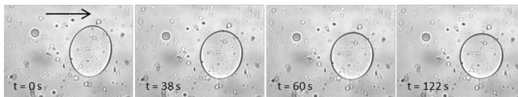
**Figure 5:** Retraction of PA drops in PBAT<sub>2</sub> matrix after drop deformation. Deformation occurred along the vorticity axis (vertical), the flow direction being horizontal (indicated by the arrow). The radius of the drop is 106  $\mu$ m.
