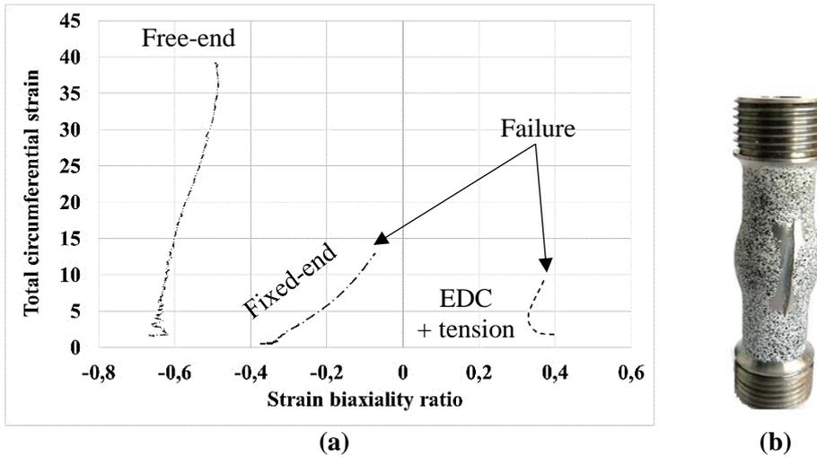
Fig. 5. Evolution of strain ratio for free-end, fixed end, and EDC with tensile load (a), failed sample after a fixed-end EDC test (b)
