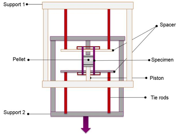
Fig. 2. EDC test with a tensile load
