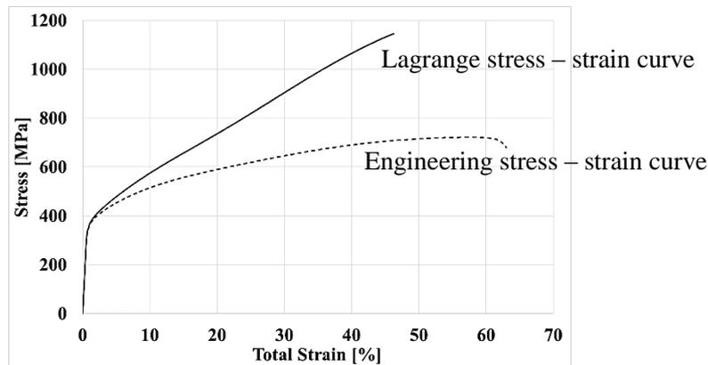
Fig. 7. Stress-strain curve for the 304L steel
