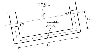
Fig. 1. Scheme of the TLCD in motion.
