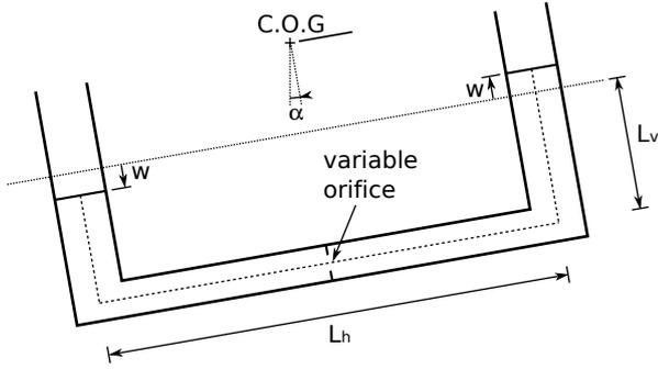
Fig. 1. Scheme of the TLCDC in motion.
