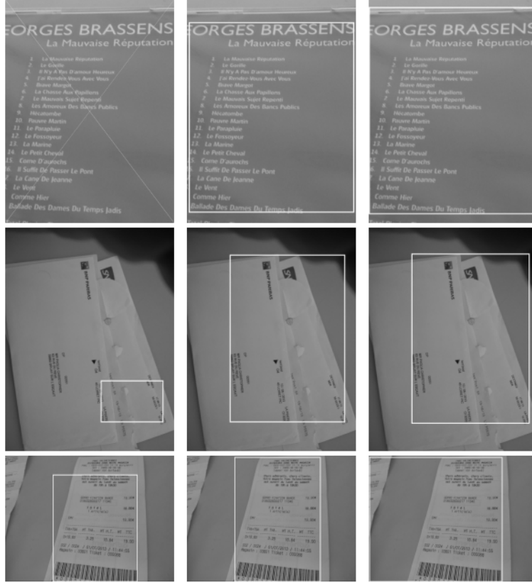
Fig. 7. Comparison between different scale sets on a subset of the LINX database. Left column: monoscale approach. Middle column: multiscale approach with scales \{1, \frac{1}{16}\} . Right column: multiscale approach with the full set of scales \{1, \frac{1}{4}, \frac{1}{8}, \frac{1}{16}, \frac{1}{32}\} .
