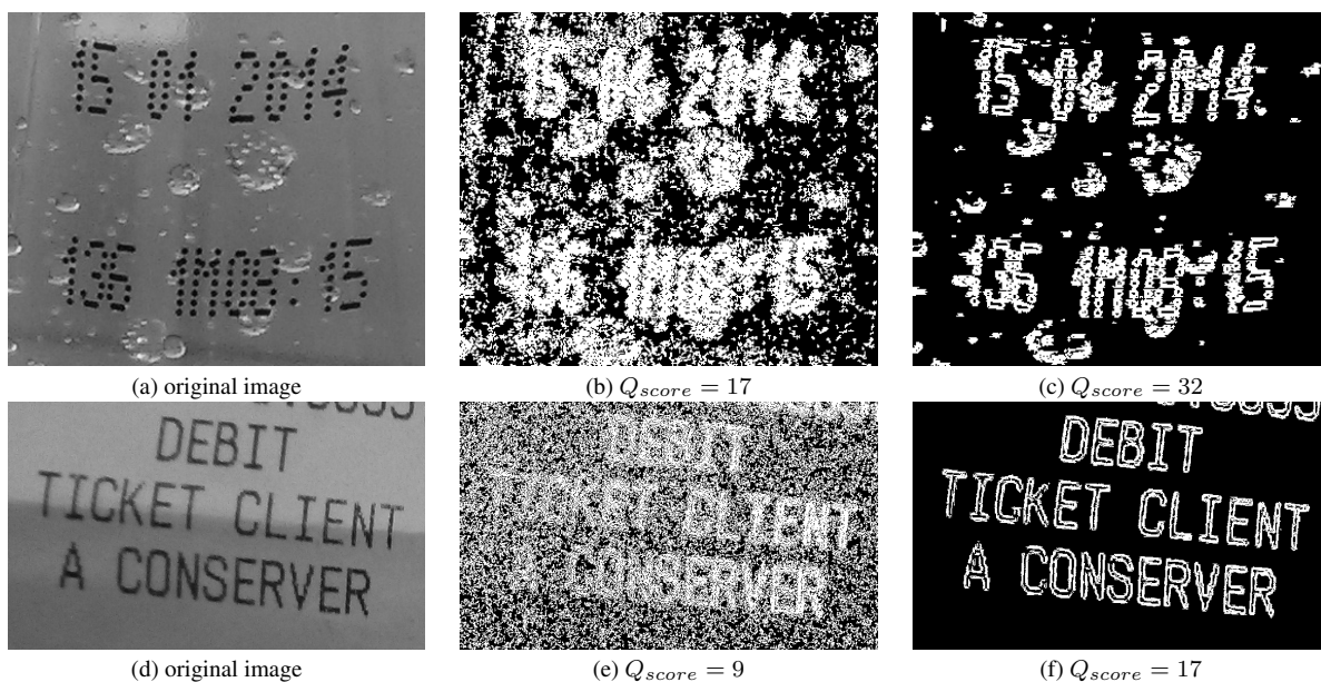
Fig. 3. Filter influence in I_Q computation. Left column: original image. Middle column: Thresholded I_Q computed from original image. Right column: Thresholded I_Q from bilateral filtered image.
