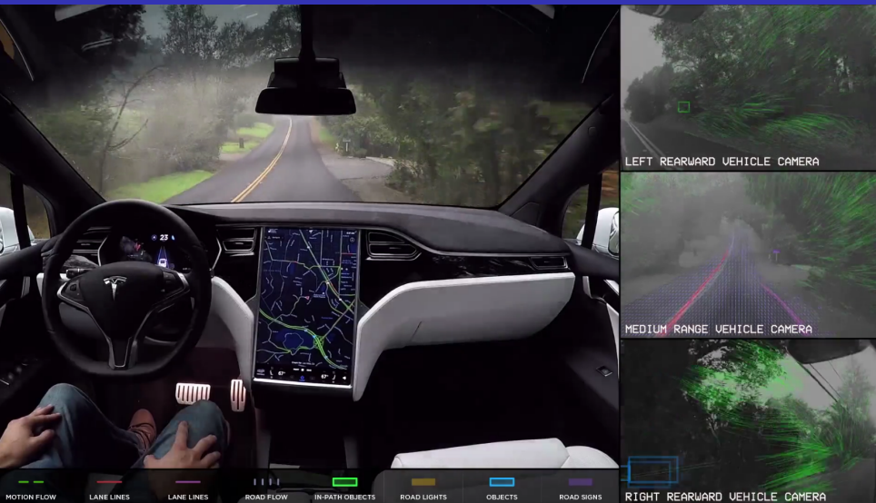
Figure: Example of motion flow analysis. Tesla Motor Company automatic drive.
