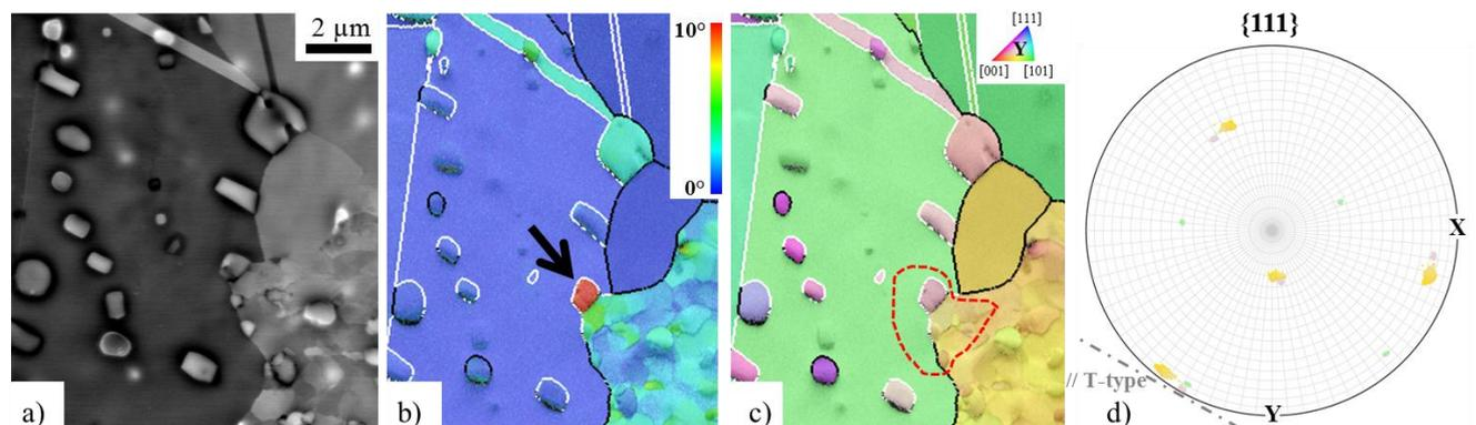
338 Fig.10 – A T-type precipitate at the recrystallization front in the AD730™ alloy (AD730™ Lab-Forged sample).
