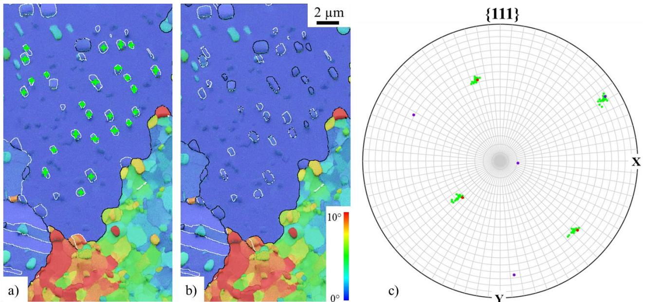
230 Fig.6 – The imperfect twin orientation relationship of the T-type precipitates (René65 billet sample). a) and b)
