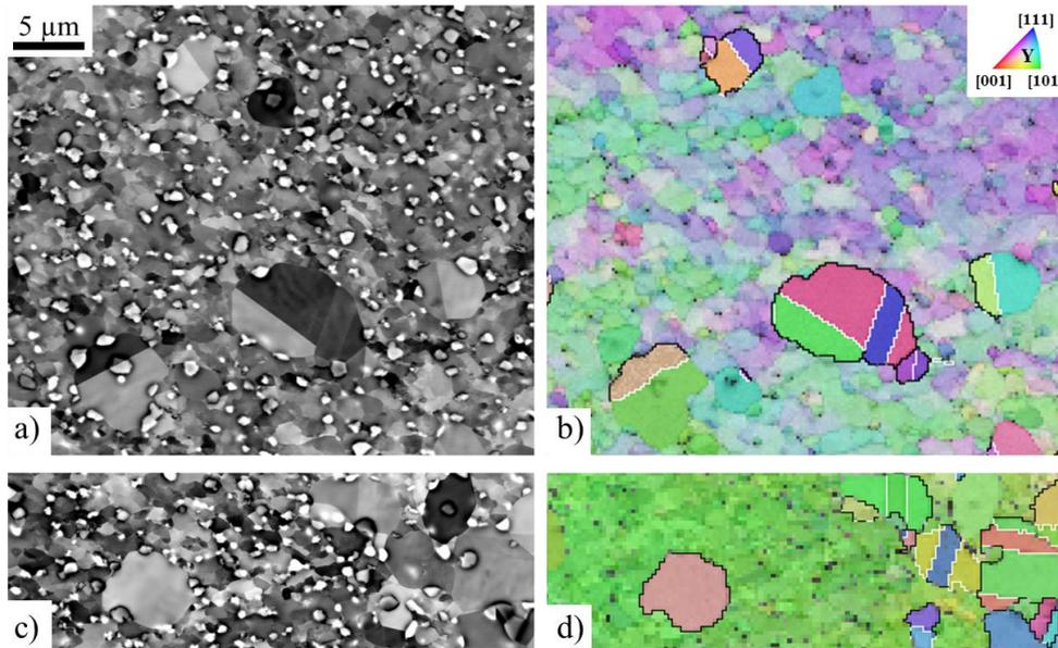
323 Fig.9 – Recrystallized grains unsuccessful in consuming the surrounding recovered grain (AD730™ Lab-Forged
