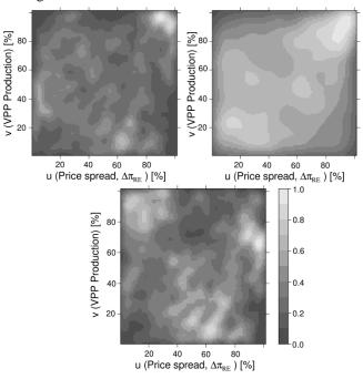
Fig. 8: Normalized density of copulas modelling dependence between price spread for revenue and VPP production:75% capacity from Wind, by KDE Copula (top left), 75% capacity from Wind, by Joe-Frank copula (1.39,0.95) (top right), 75% capacity from PV, by KDE Copula (bottom)
