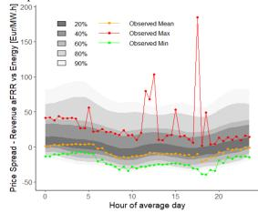
Fig. 7: Day-ahead probabilistic forecast of revenue price spread between reserve and energy, obtained by a gradient boosting tree model. Prediction intervals between 20% and 90%. Forecasts averaged at same hour of day.
