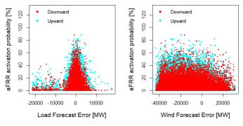
Fig. 3: Observed aFRR activation probabilities and forecast errors on load and wind production for Germany (data 2015-2016).
