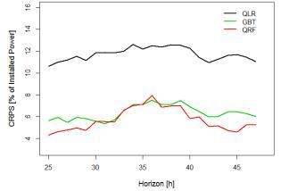
Fig. 5. Continuous Ranking Probability Score (CRPS) as a function of the forecast horizon for the QRF and the benchmarks QLR and GBT
