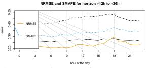
*Figure 1.* Electric demand forecast, errors and comparison with the persistence (in black)
