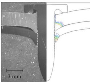
**FIGURE 1:** Experimental (Left) vs Numerical (Right) nailed-joint
