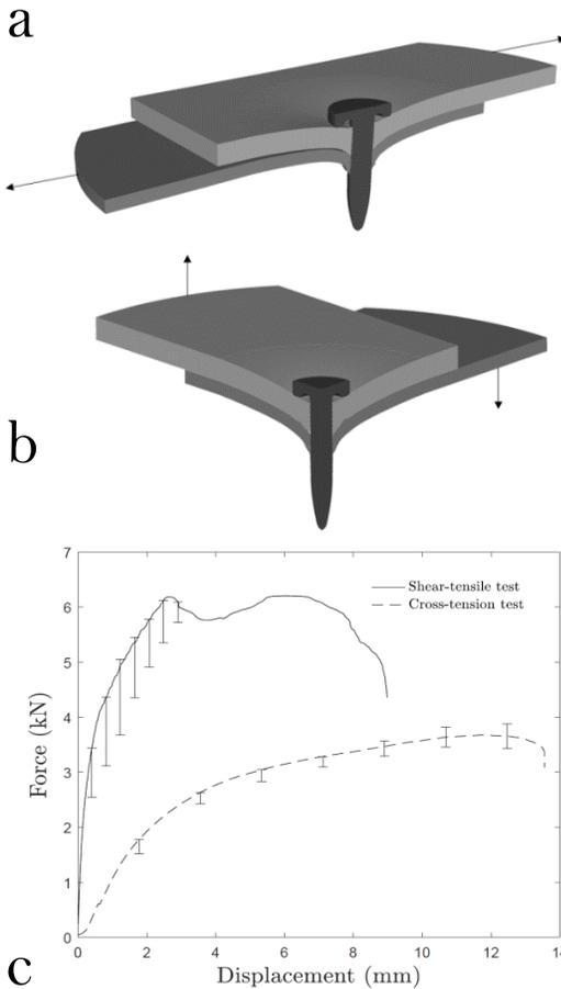
**FIGURE 2:** Cast al.(2.5mm)/DP780(1.5mm) nailed-joint
