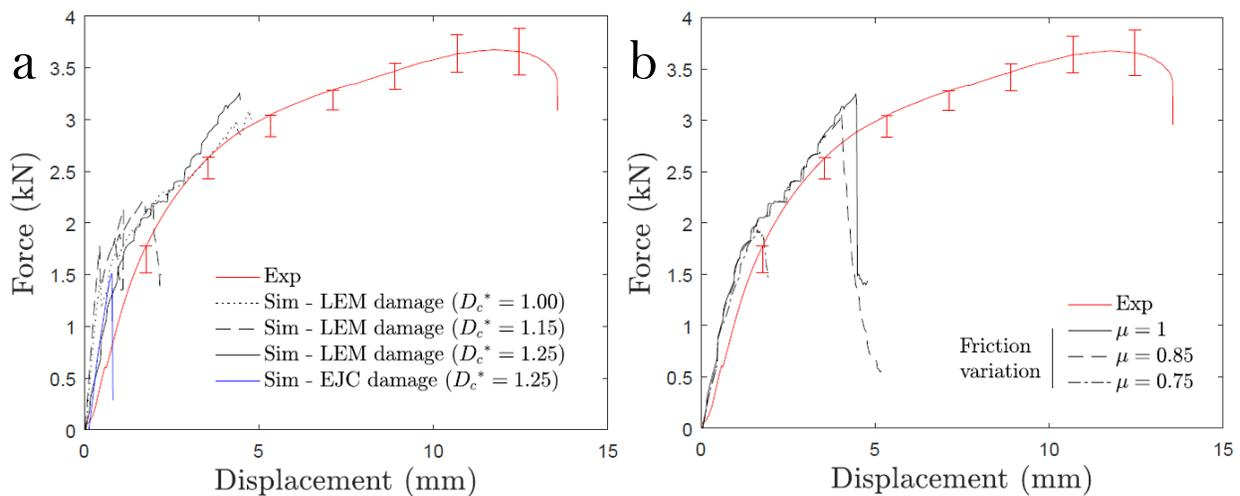
FIGURE 4: Comparisons between experimental and numerical Cross-tension tests conducted on Aluminium/Steel nailed-joint
