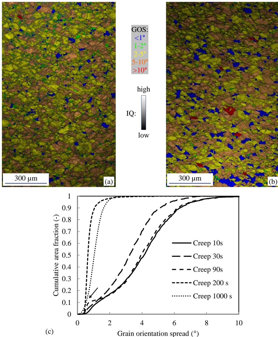
Fig. 4. Microstructural information of partially recrystallised samples at  $850^\circ\text{C}$  and 20 MPa: (a, b) combined image quality (IQ) + GOS maps after 30 and 90 sec. creep tests, respectively (the compression axis is along the vertical direction) and (c) GOS histograms for the different creep times. The arrow in this figure indicates the small fraction of recrystallised grains found in the bimodal GOS distribution after 90 s creep.
