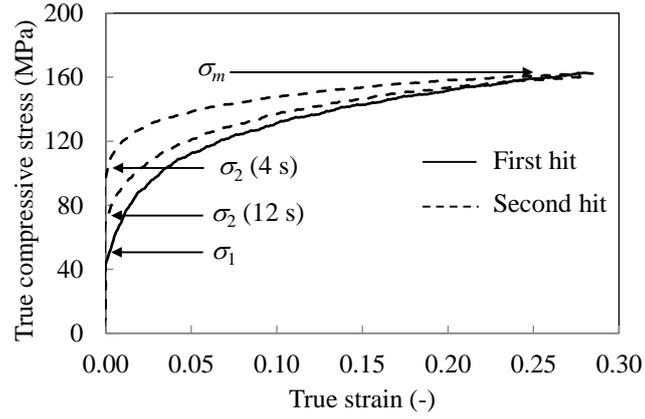
Fig. 6. Double-hit compression flow curves obtained at 950°C and with a strain rate of 0.44 s<sup>-1</sup>
