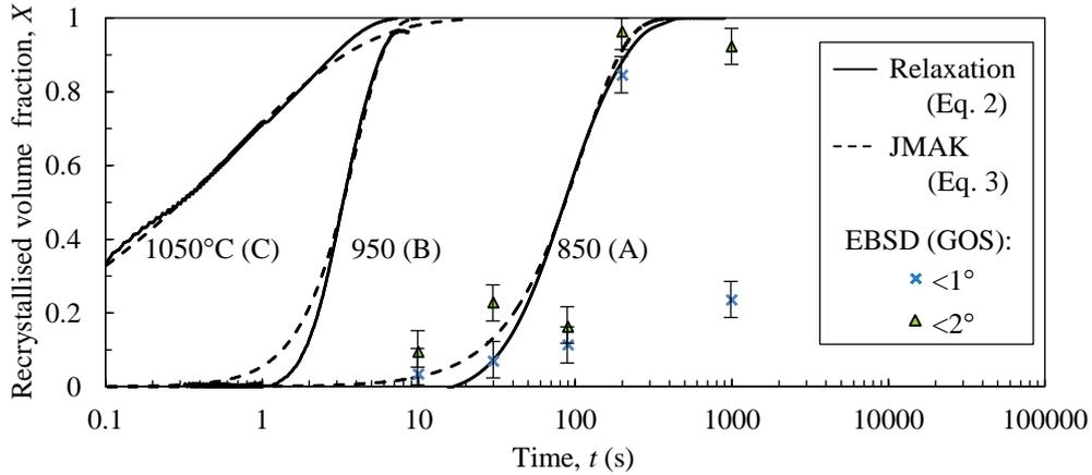
Fig. 3. A comparison between the volume fraction of recrystallised material vs. time, calculated from eq. (2) and from the JMAK relationship (eq. (3)), and measured by EBSD after interrupted creep tests
