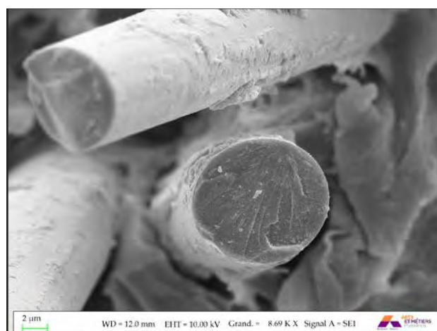
Fig. 3. Failure induced by a crossing with a neighboring fiber.
