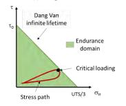
**Fig. 6.** Illustration of the Dang Van criterion The criterion is defined by the boundary between infinite life (endurance domain) and fatigue. Component life for a load path contained completely below the Dang Van Criteria line will be infinite. However, this approach does not allow to consider simultaneously low and high cycles fatigue.
