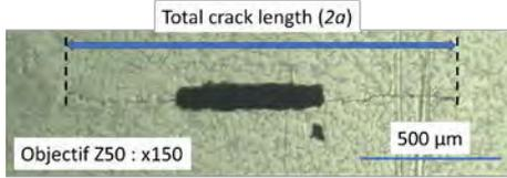
**Fig. 14.** Crack growth image analysis
