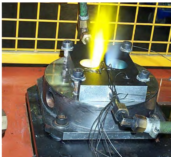
Fig. 9: Single cylinder thermal fatigue rig with an acetylene torch heating system
