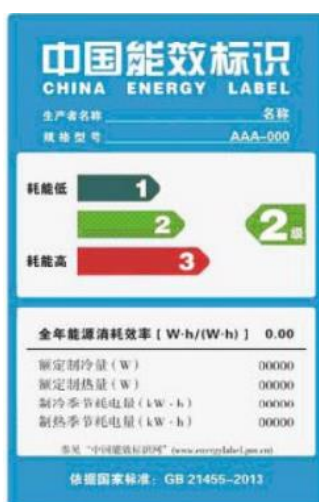
Figure 7 China Energy Label for variable speed air conditioners according to MEPS GB 21455 -2013 68
