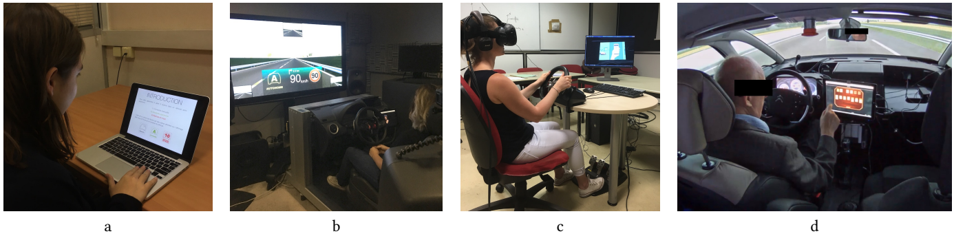
Figure 2: The three training systems: (a) the user manual displayed on the laptop computer, (b) the fixed-base driving simulator, (c) the light VR system. (d) The high-end simulator used for the test drive
