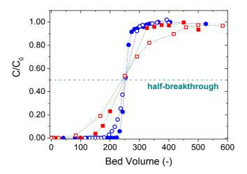
**Fig. 5.** Breakthrough curves obtained for Sorbmatech® 202 with a 1 cm diameter column, with an H/D ratio of either 5 (blue circles, T1&T2) or 2 (red squares, T3&T4) and a Darcy velocity of 2 m·h $^{-1}$  (filled symbols T1&T3) or 10 m·h $^{-1}$  (empty, T2 & T4).
