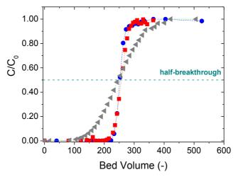
**Fig. 6.** Breakthrough curves obtained for Sorbmatech® 202 with a Darcy velocity of 2 m·h<sup>-1</sup> for different bed heights (H) and column diameters (D): blue circles, D=1 cm, H=5 cm (T1); red squares, D=2.5 cm, H=5 cm (T6); grey triangles, D=2.5 cm, H=0.8 cm (T5) (same bed volume as D=1 cm, H=5 cm).
