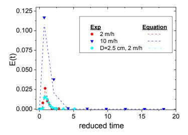
**Fig. 7.** Residence time distributions plotted as a function of reduced time, i.e. the actual time divided by the ideal residence time under continuous flow  $\tau$ , for columns (1 cm in diameter D unless specified) packed with Sorbmatech® 202 at the Darcy velocities of 2 and 10 m/h. The dashed lines are the best fits to the experimental data obtained with the model described in section 3.2 (Eq. 5).
