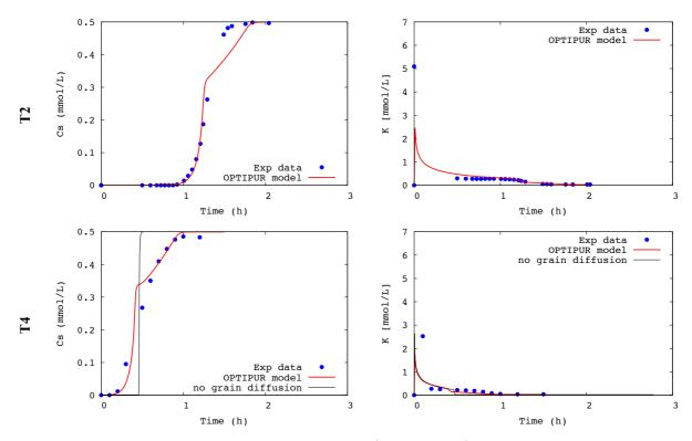
**Fig. 8.** Comparison of the breakthrough curves for  $Cs^+$  (left) and  $K^+$  (right) measured in experiments T1 (H = 5 cm, U = 2 m·h<sup>-1</sup>), T2 (H = 5 cm, U = 10 m·h<sup>-1</sup>) and T4 (H = 2 cm, U = 10 m·h<sup>-1</sup>) for Sorbmatech® 202 and calculated using the software Optipur based on the model depicted in Figs. 2 and 3.
