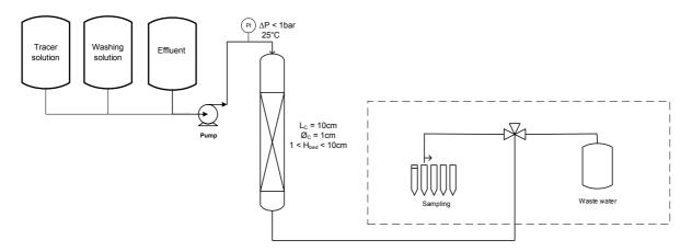
Fig. 1. Schematic diagram of the experimental set-up for the breakthrough experiments.
