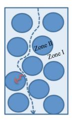
**Fig. 2.** Schematic representation of a column packed with S202 grains with the two zones in which the fluid flows by convection (dashed blue arrow, zone I) or diffusion takes place only (solid red arrow, zone II).
