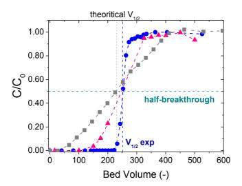
**Fig. 4.** Breakthrough curves obtained for Sorbmatech® 202 with a 1 cm diameter column, with a Darcy velocity of 2 m·h<sup>-1</sup> and bed heights of 5 cm (blue circles, T1), 2 cm (magenta triangles, T3) or 0.39 cm (grey squares, T7).
