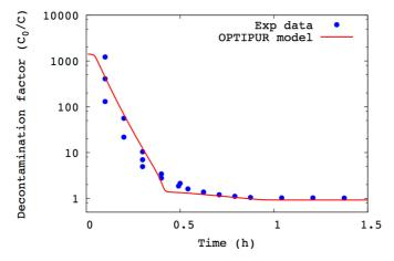
**Fig. 9.** Comparison of the decontamination factors measured in experiment T4 (H = 2 cm, U = 10  $\text{m} \cdot \text{h}^{-1}$ ) for Sorbmatech® 202 and calculated using the software Optipur based on the model depicted in Figs. 2 and 3.
