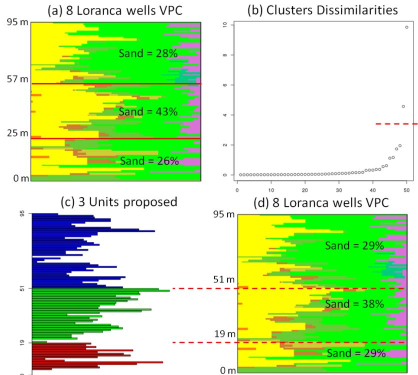
**Figure 5** Illustration of real data test, 8 Loranca wells. (a) VPC of 8 Loranca wells, plain red lines show 3 units proposed by geologists; (b) Clusters Dissimilarities graph, the 3 last clusters considered as the most dissimilar. (c) The sand part of VPC (3 last clusters). (d) VPC of 8 Loranca wells, red dotted lines show the 3 simulation units proposed by clustering.
