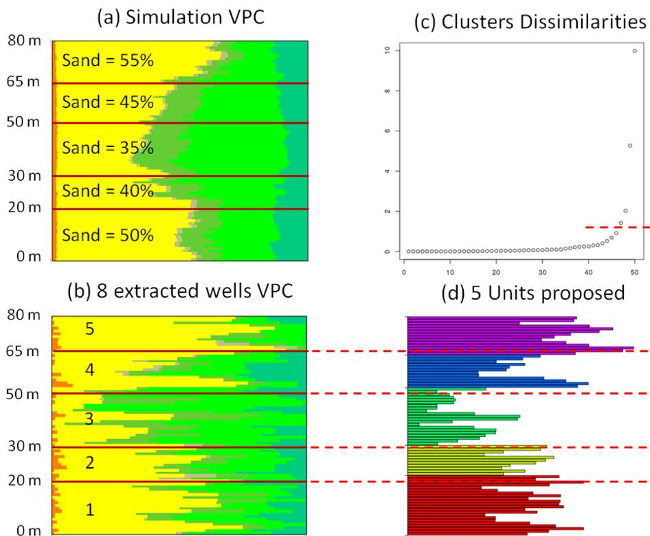
**Figure 4** Illustration of synthetic test, Flumy simulation with less contrasted units. (a) Simulation VPC, red lines represent the limits between the initial units. (b) VPC of 8 extracted wells. (c) Clusters Dissimilarity graph; the 5 last clusters are the most dissimilar. (d) The sand part of VPC, the colors correspond to 5 last clusters.
