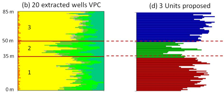
**Figure 3** Illustration of synthetic test, Flumy simulation with contrasted units. (a) Simulation VPC, red lines represent the limits between the initial units. (b) VPC of 20 extracted wells, the initial units are hardly detectable by a visual criterion. (c) Clusters Dissimilarities graph; the 3 last clusters are the most dissimilar. (d) The sand part of the wells VPC, the colors correspond to the 3 last clusters.
