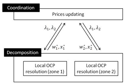
Fig. 1. Decomposition-coordination algorithm
