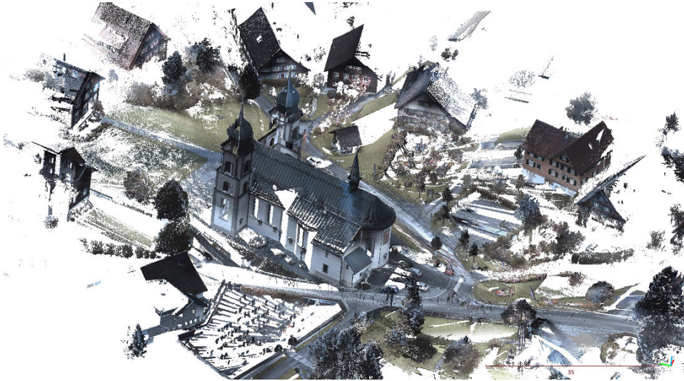
Figure 3: Exemple of cloud in Semantic3D dataset (3 clouds registered). Occlusions, density depends on the distance to the LiDAR.
