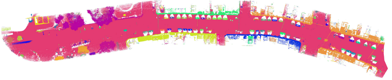
Figure 9: Example of cloud segmented by our method (each object has a different color).
