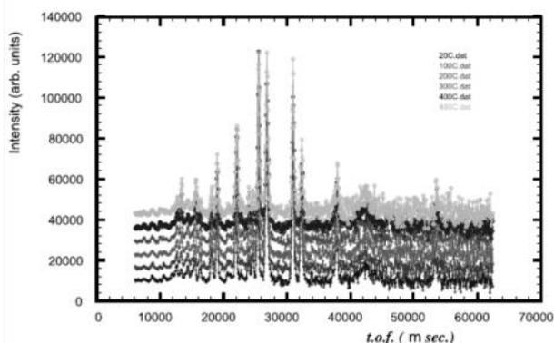
**Fig. 7.** Successive TOF patterns taken at stabilized temperatures in increasing order (in °C): 20, 100, 200,300, 400, 480. The patterns are vertically shifted to improve visibility.
