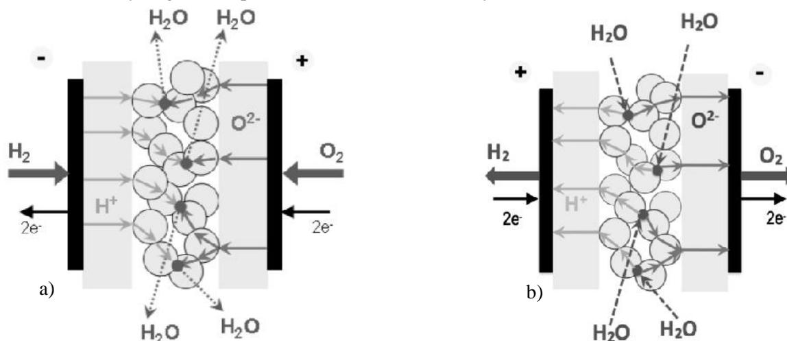
**Fig. 1.** Schematic representation of the reversible dual membrane fuel cell concept based on a single mixed ion conduction material: a) fuel cell mode of operation; b) electrolyzer mode of operation.
