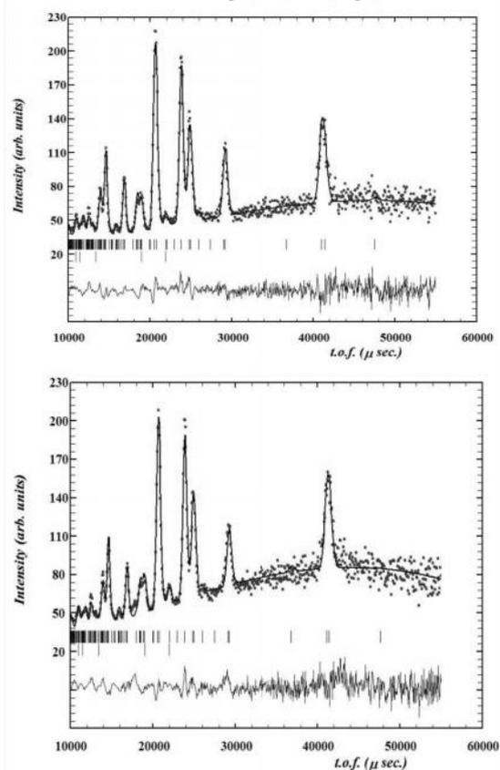
**Fig. 6.** Observed (crosses), calculated (continuous line), and difference (bottom) Rietveld ND profiles at 295 K. Left: BCY15 based pellet; Right: as received BCY15 powder without temperature treatment. The row of tick marks gives the positions of the allowed Bragg reflections.
