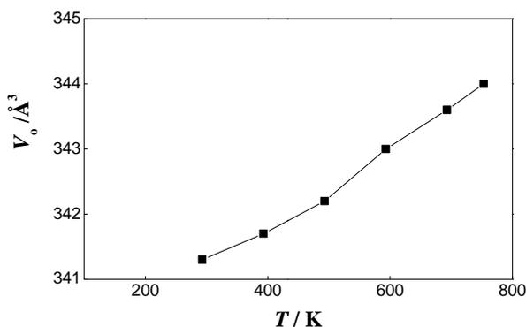
**Fig. 9.** Temperature dependence of unit cell volume  $V_0$  of BCY15 pellet of 13% porosity.
