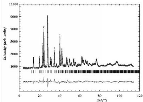
**Fig. 5.** Observed (crosses), calculated (continuous line), and difference (bottom) Rietveld ND profiles of milled material of dense BCY15 pellet at 295 K. The row of tick marks gives the positions of the allowed Bragg reflections.
