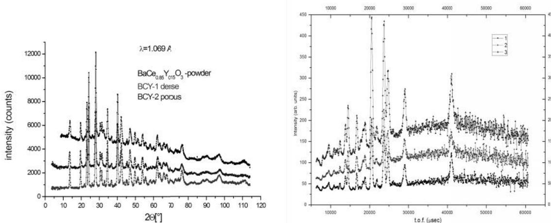
**Fig. 4.** ND patterns of BaCe<sub>0.85</sub>Y<sub>0.15</sub>O<sub>3</sub> based samples at 295 K: a) constant wavelength ( $\lambda = 1.069 \text{ \AA}$ ) pattern. The sample denoted as powder was kept for three days in moist air; b) TOF patterns: 1 (dense), 2 (porous), 3 (powder). The patterns are vertically shifted to improve visibility.
