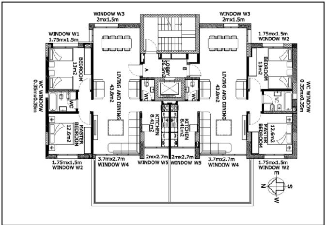
FIGURE I PLAN VIEW OF BUILDING'S TYPICAL FLOORS (WITH TWO APARTMENTS A AND B)
