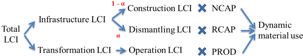
Figure 2. Disaggregation method and coupling of technologies' LCIs to the TIAM-FR outputs
