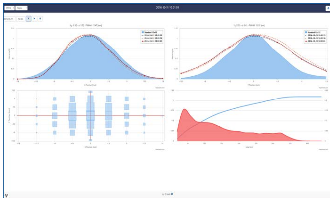
Fig. 8. Beam profile display. In the upper part, the X-Y Gaussian profiles of the beam are displayed. In the bottom part (left-hand side), one sees the pad intensities while on the right-hand side, the longitudinal profile of the beam.
