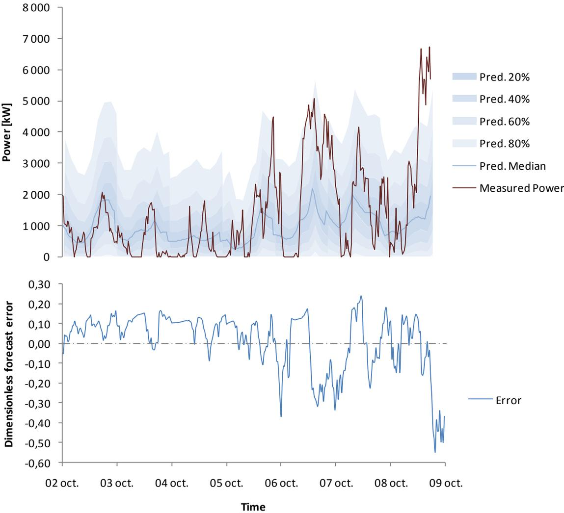
**Figure 4: (a) Prediction of wind power production showing the quantiles of the prediction probability distribution, its median and the observed production in the same period. (b) Dimensionless error between observed wind power production and its day-ahead prediction. The diagrams are relative to the period 02-08/10/07**
