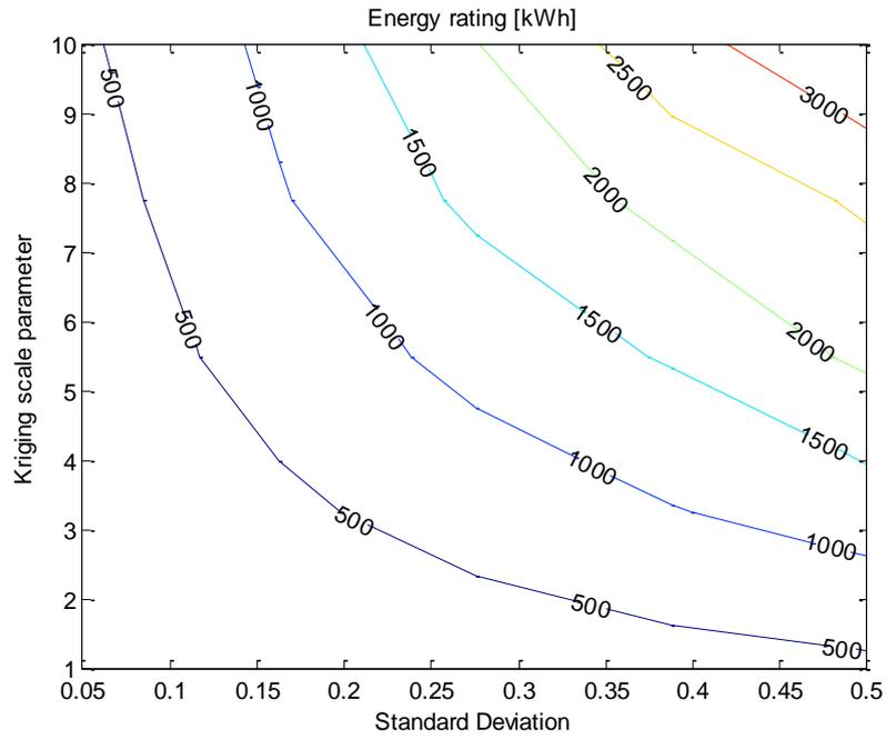
Figure 7: Optimal storage energy rating for different values of prediction errors standard deviation and autocorrelation
