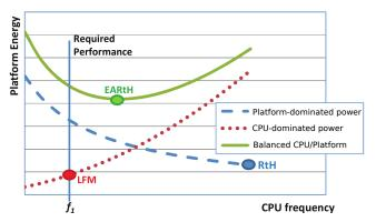
Fig. 1. Conceptual view of platform energy consumption by Rotem et al. [5].
