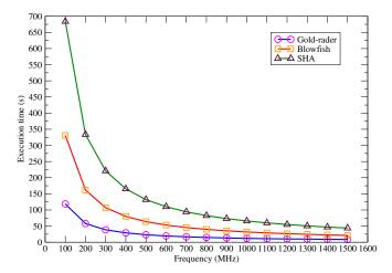
Fig. 6. Execution time vs. Frequency: performance of the benchmarks with varying clock frequency on the TI AM572x platform.
