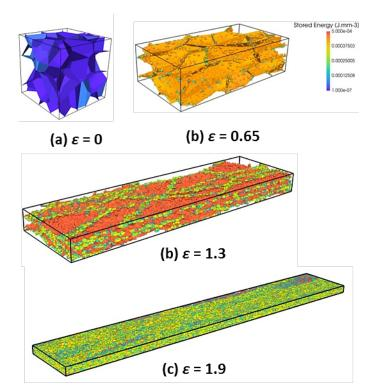
Figure 1. Simulation of a channel-die compression of the 304L steel at 1000°C and at a strain rate of 0.01s-1. Four different instants are represented: (a)  $\varepsilon = 0$ , (b)  $\varepsilon = 0.65$ , (c)  $\varepsilon = 1.3$ , (d)  $\varepsilon = 1.9$ . The initial number of grains is 64 and the final number of grains is around 50.000.
