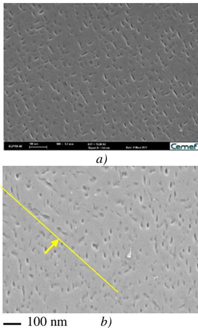
Figure 2: SEM secondary electron image providing the  $\gamma''$  phase topology in aged samples (500 h @ 650 °C)
