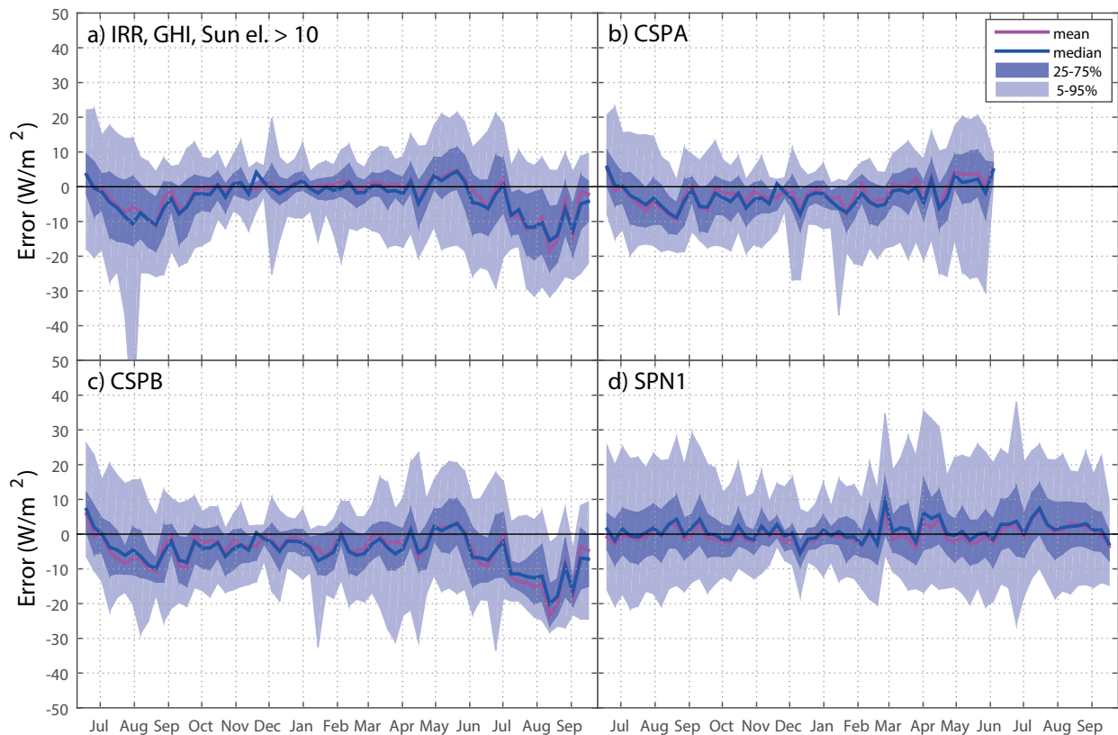
Figure 3: Mean, median, interquartile range and 5–95 percentile range of weekly error distribution between tested and reference instrument for GHI.
