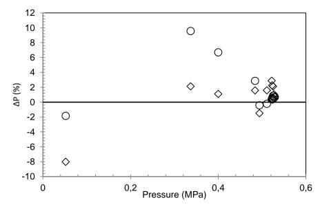
Figure 5 : Percentage error (BIAS) in the prediction of VLE pressure for the n-butane – methanol system at 323.2 K. [18].  $\diamond$  GC-PR-CPA EoS.  $\bigcirc$  PR78-MHV2-UNIFAC model
