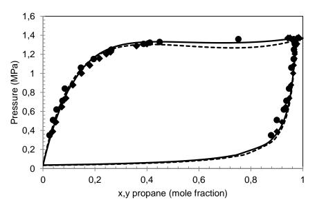
Figure 2 : Phase equilibria of the propane – methanol system at 313.01 K. ◆ [2] and ● [13]. Solid lines: GC-PR-CPA model. Dashed lines: PR78-MHV2-UNIFAC
