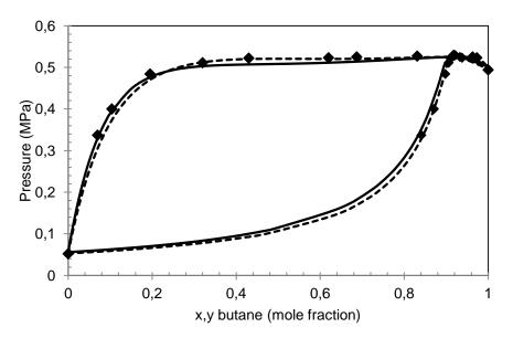
Figure 3 : Phase equilibria of the n-butane – methanol system at 323.2 K. [18]. Solid lines: GC-PR-CPA model. Dashed lines: PR78-MHV2-UNIFAC
