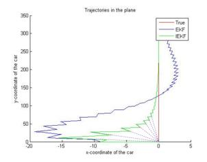
Fig. 2: First numerical example of Theorem 1: True, IEKF and EKF estimates trajectories of a car with perfect odometry, known initial position and uncertain initial heading. The odometry indicates  $\omega_t \equiv 0$ , thus the car is necessarily moving along a ray emanating from its original position. The IEKF encodes correctly this information, as its estimates always move along rays emanating from the initial position indeed.
