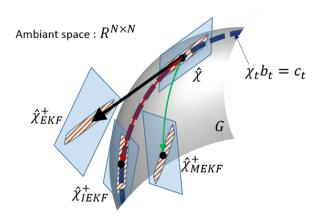
Fig. 1: Schematic difference between the EKF, the MEKF and the IEKF updates, illustrating Theorem 1. The dotted curve represents the subgroup (11), and the hatched areas the covariances, originally consistent with (11). The IEKF stays on the subgroup, while the MEKF and the EKF update respectively leave the subgroup and even the group G.
