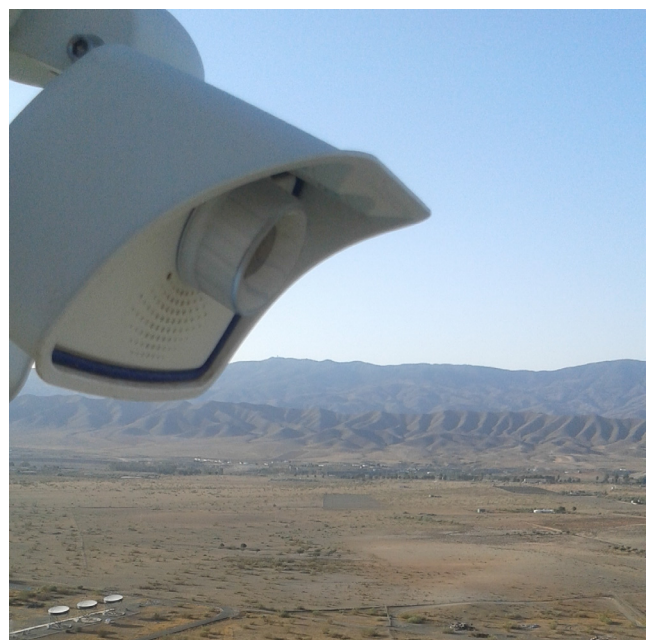
Fig. 1. One of the six shadow cameras overlooking the PSA from top of a tower.
